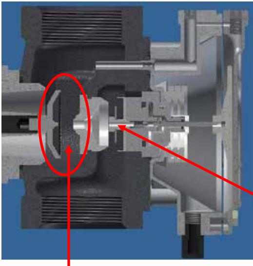
Under normal operational conditions, the P303 Series performs as the P300. When there is a demand downstream of the regulator, the main valve disk moves away from the orifice to allow flow. The Monitor diaphragm and piston are always in motion based on outlet feedback through the pitot tube at the outlet.
