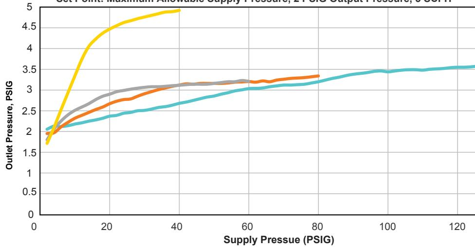
— 0.25" Orifice — 0.375" Orifice — 0.5" Orifice — 0.75" Orifice
