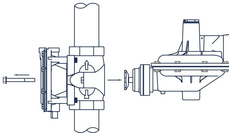
1. REMOVE BOLTS AND P303 FROM BODY, AND REMOVE FROM LINE.
