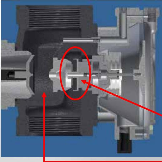
The monitor module will activate when the system experiences a failure such as the main valve disk is stuck open or the lever disengages from the valve stem assembly. When the P303 main regulator fails to regulate and the output pressure climbs, the increased output pressure will move the monitor valve disk towards the secondary sealing surface of the orifice.
