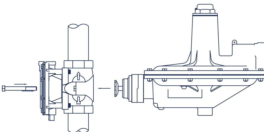
2. USE BOLTS SUPPLIED WITH HEAD ONLY VERSION TO ATTACH TO BODY ALREADY INSTALLED.
