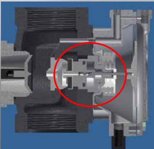
Once the output pressure has increased 7" to 28" WC above the set operating output pressure, the monitor valve disk will fully seal on the secondary sealing surface of the orifice. At this point, the only supply pressure that is passing through the unit is passing through the tiny bleed hole on the disk holder screw and venting directly out the main regulator diaphragm assembly and through the main regulator's vent assembly.
