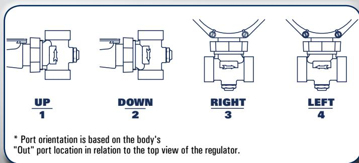
\* Port orientation is based on the body's "Out" port location in relation to the top view of the regulator.
